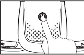
1. Gently press the on/off button to turn off the drone.
