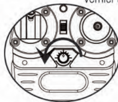
Counterclockwise rotation vernier adjustment knob
