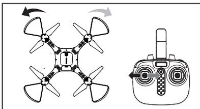
When the left joystick (throttle) is pushed towards the left or right, the drone will turn left or right correspondingly.
