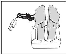
3. Insert the USB port of USB charging cable to power supply and the red indicator light will turn on, while the battery is inserted for charging the green indicator light will turn on, and it will turn off when charging completed. It takes about 150 minutes to completely charge the battery.
