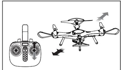
When the right joystick (rudder) is pushed upwards or downwards, the drone will fly forward or backward correspondingly.
