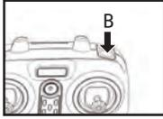
Method 3: When the drone is stationary, press the button B, the drone automatically takes off and hovers at a certain height.
