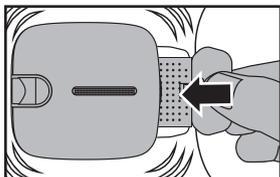
4. After charging completed, replace the battery into the drone.
