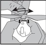
Press the blade lock down, and then the blade "A" is rotated in A clockwise direction to remove, and it is locked in A counterclockwise rotation; The blade B is rotated in A counterclockwise to remove, and it is locked in A clockwise rotation.
