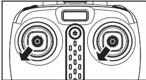
When the drone encounters a direct impact with foreign objects in the headless mode, if there is an occurrence of deviation of the defined direction, it is only required to push both the left and right joysticks to the bottom left corners simultaneously after placing the flying direction of the drone in the correction position. When the led light indicator of the drone is in a long “ON” mode after slowly flashing for 3 seconds, it indicates the calibration
