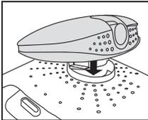
1. Connect the camera's wire connector to the drone.
