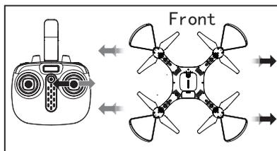
When the right joystick (rudder) is pushed towards the left or right, the drone will fly sideways on the left or right correspondingly.
