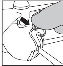
1. Insert the protective gear into the two jack connectors underneath the main body as shown in Figure 1.
