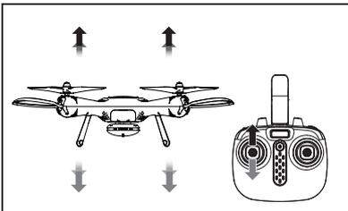
When the left joystick (throttle) is pushed upwards or downwards, the drone will ascend or descend correspondingly.
