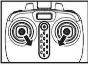
Method 2: Push the left and right joysticks to the bottom inner corners for 1 second, the blades of the drone start rotating slowly.
