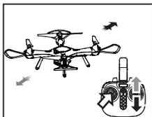
If the drone automatically flies forward/backward while hovering, press in the left joystick and at the same time push the right joystick backward/forward slightly to fine tune the direction. Don't release the left joystick until the drone is flying in a stable state.
