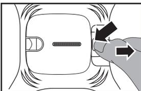
2. Press the fixed components at the bottom of the battery and pull out the battery.
