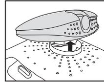
2. Take out the camera upward and disconnect the wire connector from the drone.
