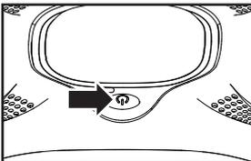
1. Press the power button on the top of the drone to make sure the drone is turned "OFF".
