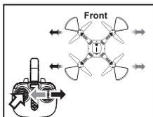
If the drone automatically flies towards the left/right side while hovering, press in the left joystick and at the same time push the right joystick right/left slightly to fine tune the direction. Don't release the left joystick until the drone is flying in a stable state.
