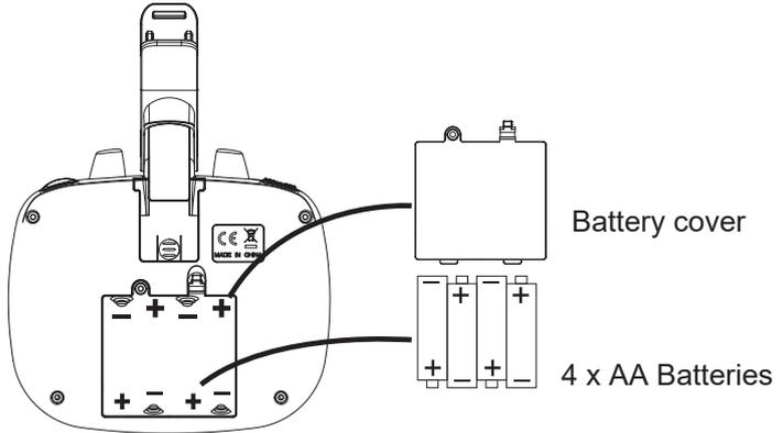
**Battery Installation Method:** Open up the battery cover at the back of the remote control. Correctly place 4 x AA alkaline batteries in the battery box in strict adherence to the polarity instructions ( batteries are not included).
