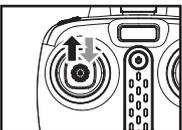
Method 1: Push the left joystick (throttle) to the highest point and then back to the center, of the drone the blades start rotating slowly.
