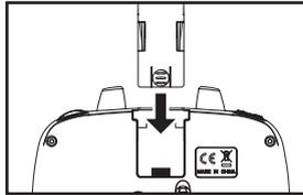
2. Insert the phone clip holder into the connector at the top of the remote control.
